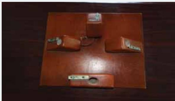
**Figure 2:** A square board measuring 16 by 16 inches in length and width with 4 wooden blocks placed on each of the four sides. Each of the four wooden blocks has a hole in the upper one third that bears a wooden pole. Each of the wooden blocks is inclined at 60° to the floor of the wooden square.
