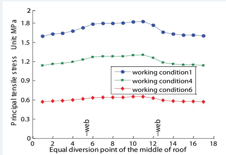
Figure 17: Middle of Zero block stress improvement.
