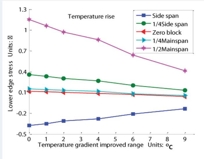
Figure 6: Superior margin stress of Temperature rise.
