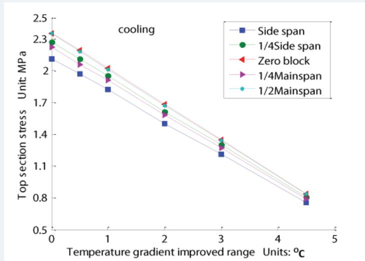
Figure 7: Superior margin stress of Temperature drop.
