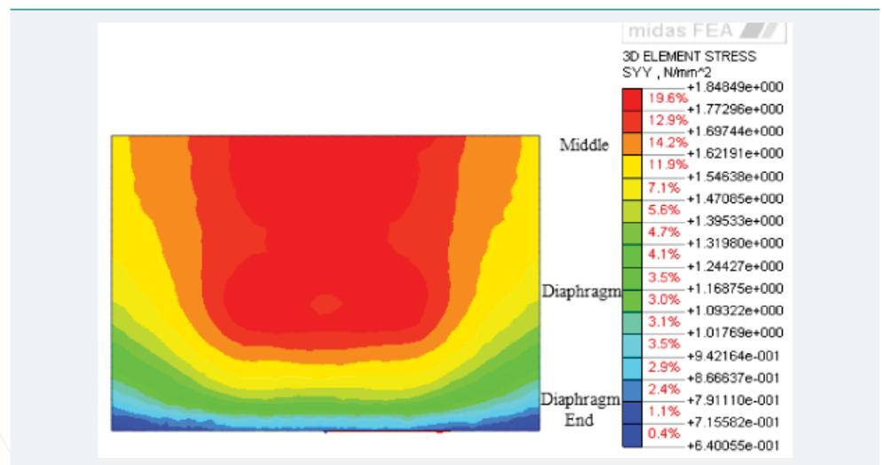
Figure 12: Longitudinal stress of roof under cooling.
