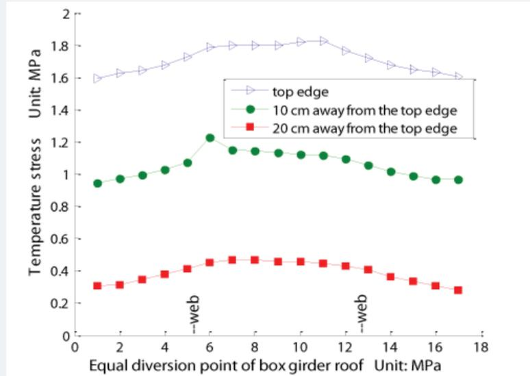
Figure 16: Principal tensile stress along roof.
