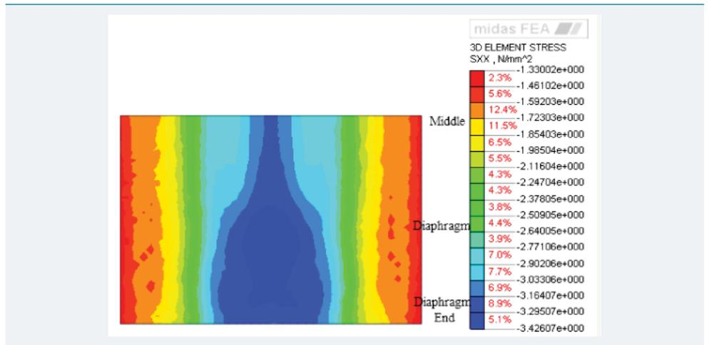
Figure 9: Transverse stress of roof under rise.
