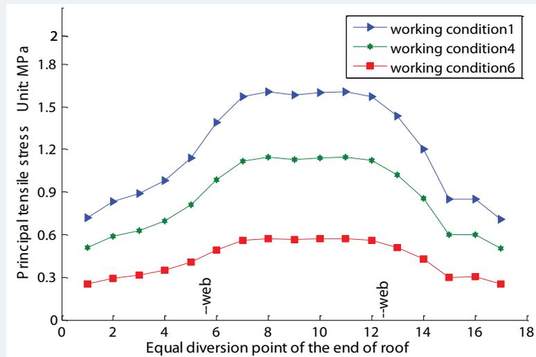
Figure 18: End of Zero block stress improvement.
