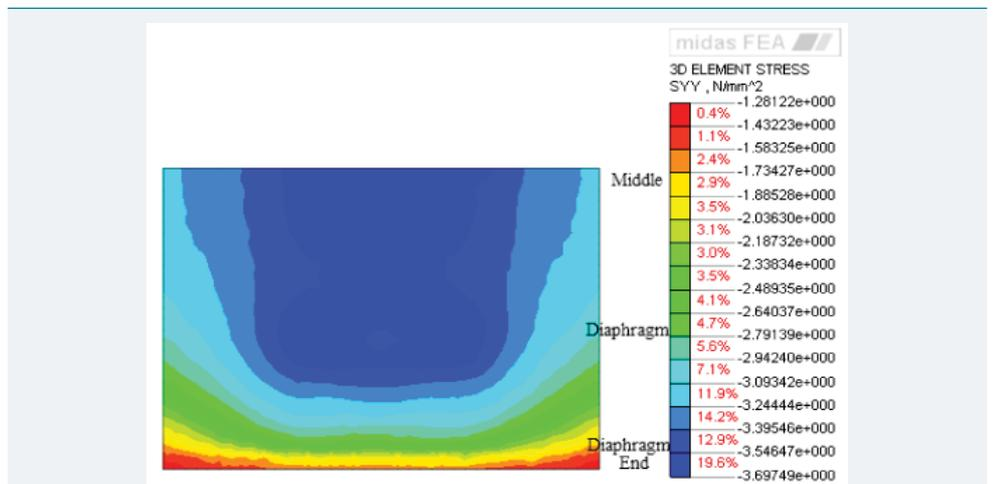
Figure 10: Longitudinal stress of roof under rise.
