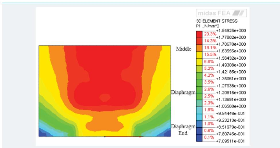
Figure 14: Principal tension stress of roof.
