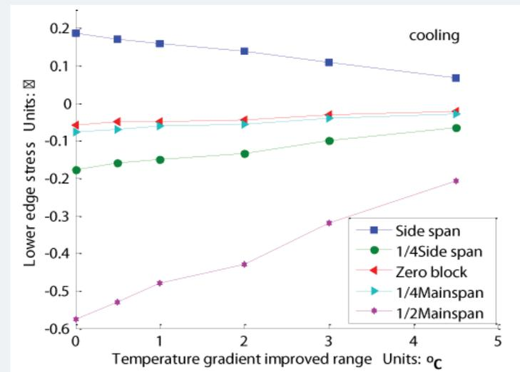
Figure 8: Lower margin stress of Temperature drop.
