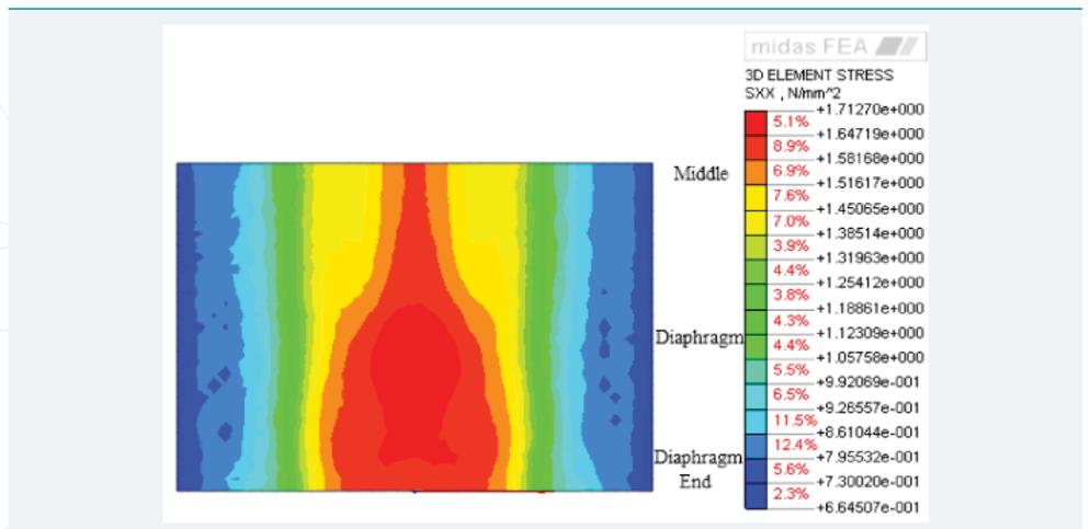
Figure 11: Transverse stress of roof under cooling.
