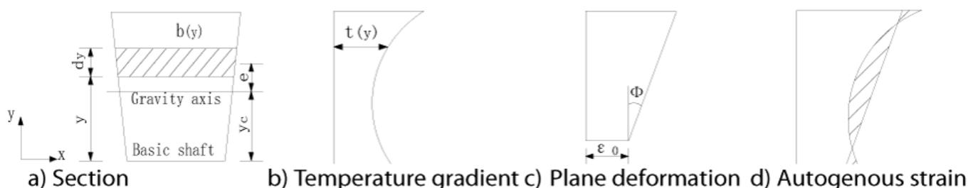
**Figure 1:** The mechanism of temperature effect. Figure a) shows position of the sectional characteristic, the shaded part is the micro units of the studied temperature effects, Figure b) shows the mode of temperature gradient, Figure c) for the assumption of plane deformation section, Figure d) shows the temperature strain superposition of the vertical and horizontal bridge.
