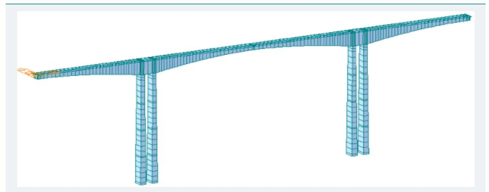
Figure 2: The whole bridge finite element model.
