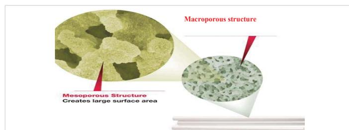
Figure 6: Structure of monolithic stationary phase.
