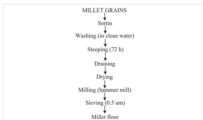
Figure 1: Flow chart for the production of millet flour. Source: Sengeve, et al. [14]
